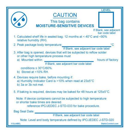
This SCS 113Label is a 4" by 4" mositure sensitive caution label. This label can be used on moisture barrier bags to identify moisture sensitive devices for levels 2, 2a, 3, 4, 5, and 5a as defined by J-STD-020. The strong, permanent adhesive is for one-time use. A total of 100 labels per roll. Roll core size 3" diameter.
